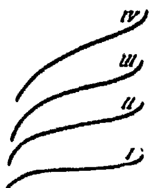
FIG. 1 Concentration gradient after different time periods. (Photometric determination of the Tyndall-cone on the surface between solution and solvent.)
